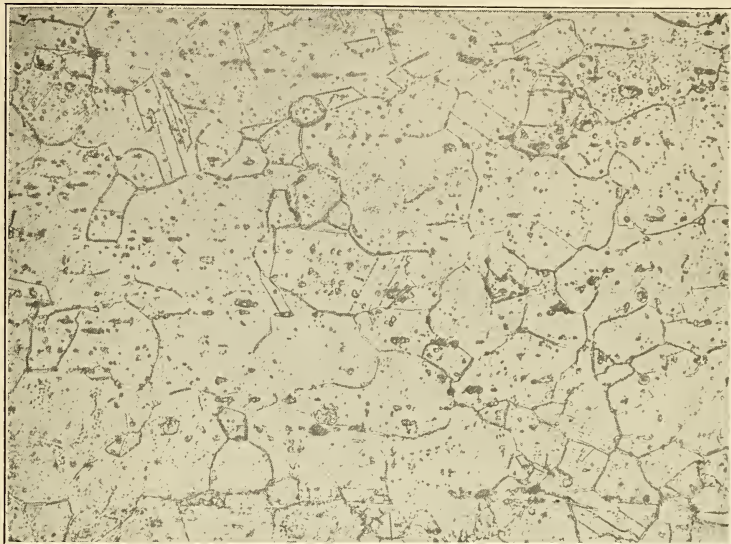
FIG. 14.—Longitudinal section of copper cylinder annealed at 650° C. Spot is located near one of the bases of the cylinder and very near its periphery. \times 200
